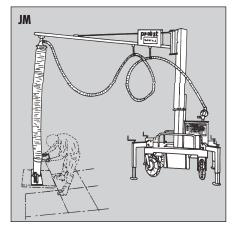
Vacuum Slab Laying Machine JUMBOMOBIL JM
